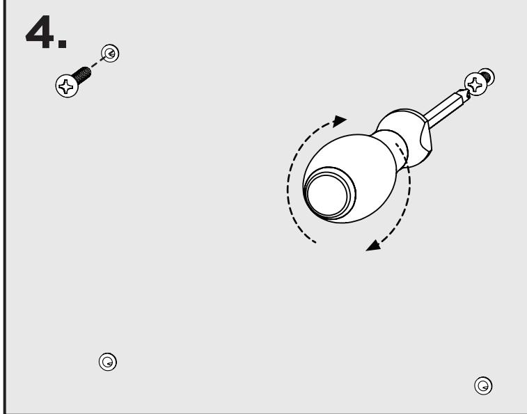
**4. Hand screw in 2 of the provided screws into the top 2 anchors only. Leave the screws out about 1/4" to allow the head of the screws to slide into the top keyholes on the back of the dispenser.**
