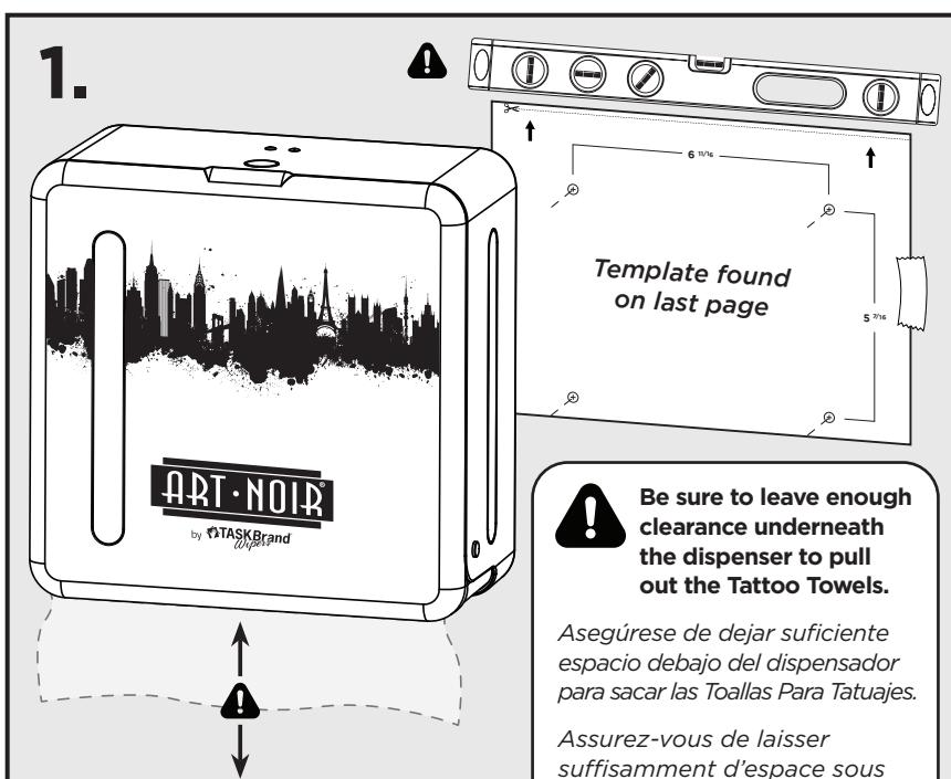
**1. Cut out Wall Mounting Template from the last page of these instructions. Tape the provided template to the wall where the dispenser will be mounted.**
