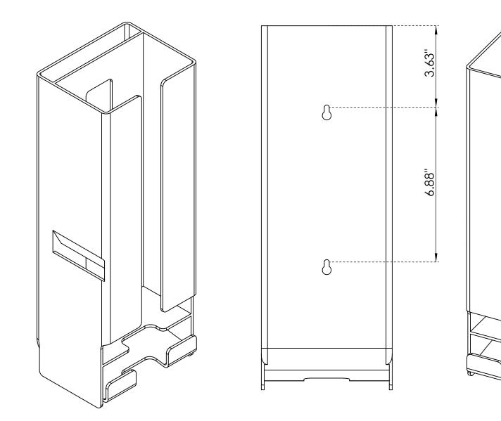
Can be mounted to the wall with screws or double sided tape, or can be placed on a flat surface.
